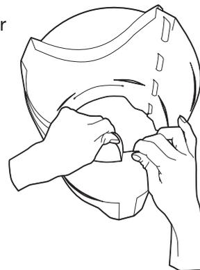
05. Insert the light bulb assembly through the lower part of the lamp.
