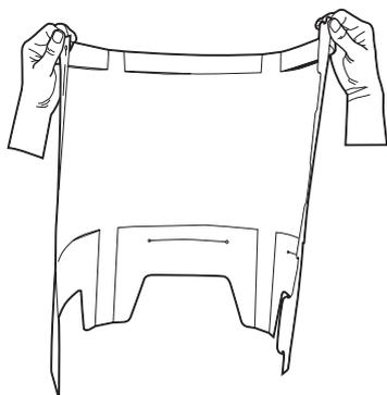
02. Insert each flap through its corresponding slot from outside to inside.
